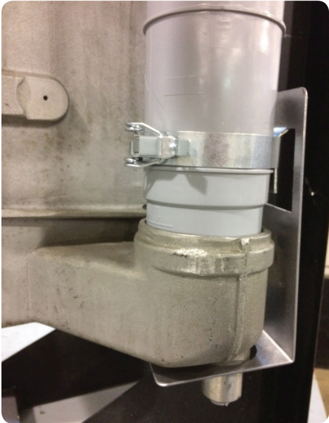
Figure 12 Offset flange of L bracket, clamp in place
